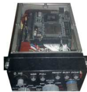
Figure 1.4 (a) AH-64A helicopter, (b) Sensor locations in an AH-64A monitored by the MSPU, and (c) Exposed-top MSPU unit [13]
