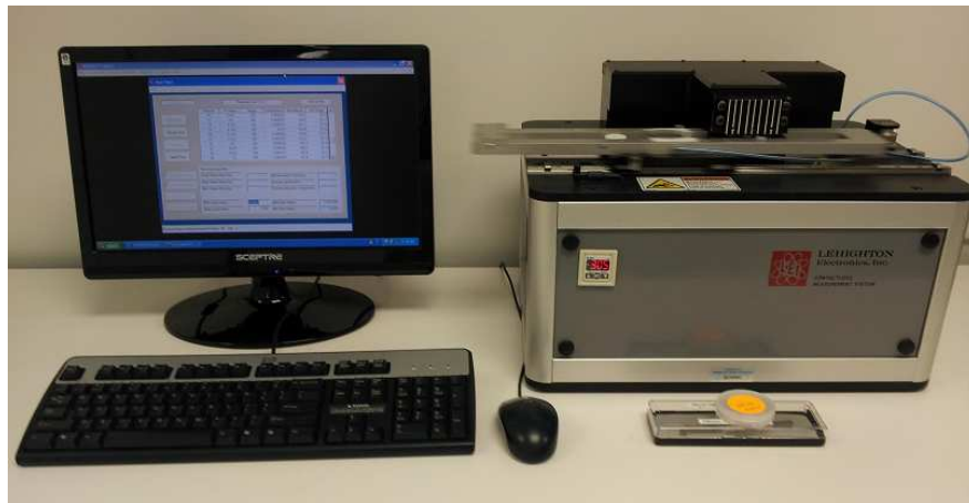
Figure 3.13: Sheet resistance mapping setup LEI 1510
