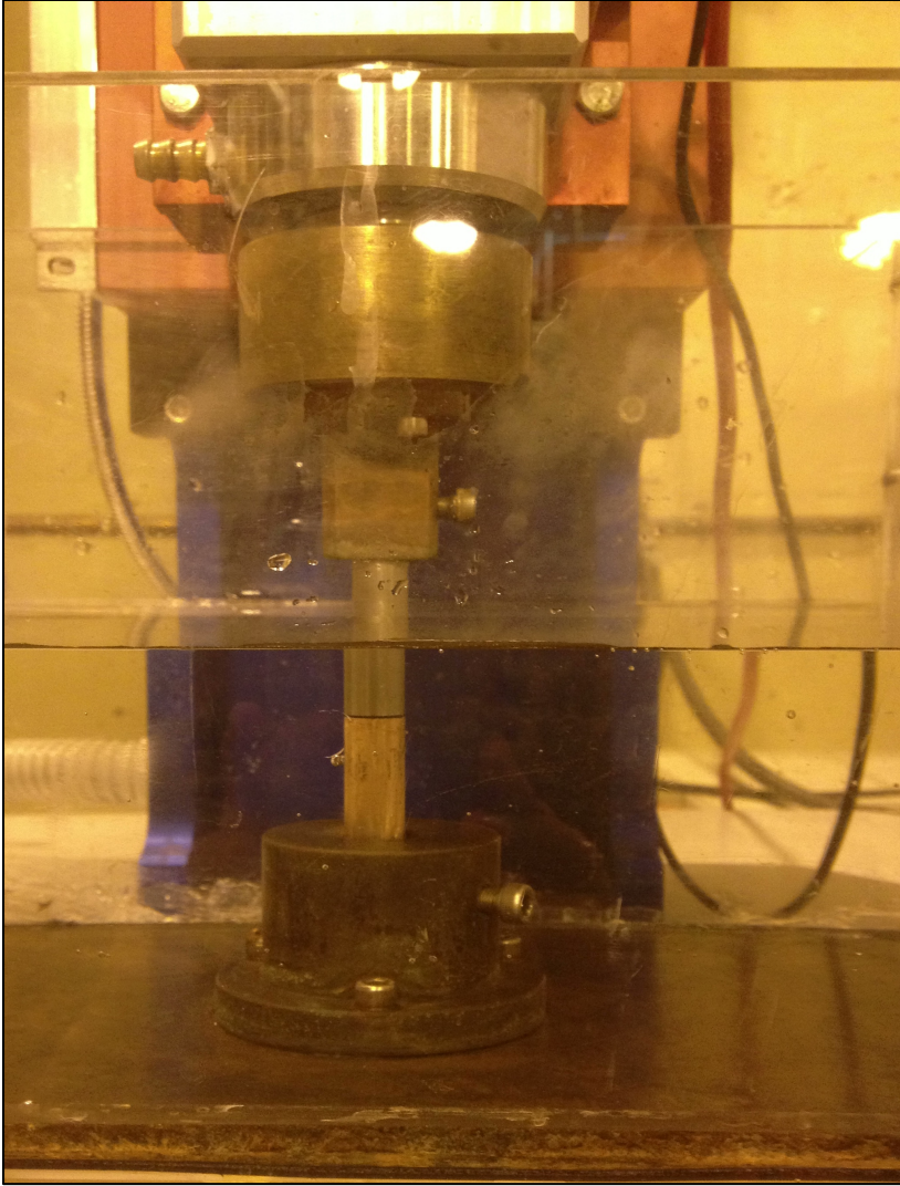
Figure 4.2: Electric discharge setup. The steel work-piece rotates while the copper tool electrode is anchored to tank base.
