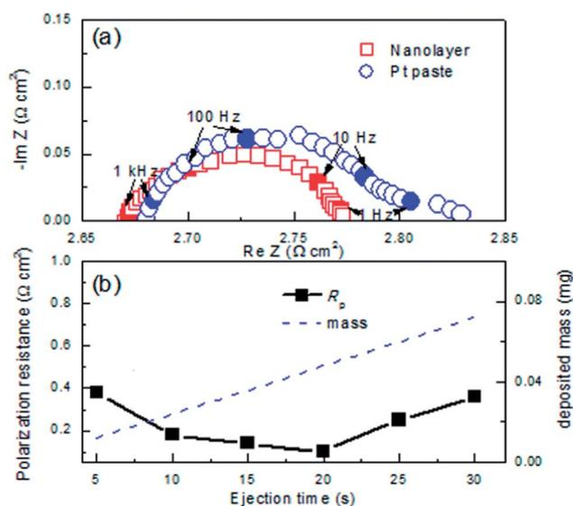
Fig. 2 (a) The Nyquist plots of symmetric cells with composition of PBCO/SDC/PBCO with different types of current collectors at 650 °C; (b)  $R_p$  vs. ejection time (sprayed platinum nanoparticle mass) at 650 °C.
