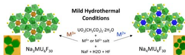
Figure 6. Mild hydrothermal crystal growth of \text{Na}_x\text{MU}_6\text{F}_{30} showing the structures and representative crystal pictures for each compound.
