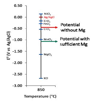
Figure 2. Electrochemical potential for alloy components and Mg corrosion inhibitor
