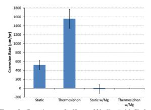
Figure 3. Corrosion rate for Haynes 230 alloy in MgCl<sub>2</sub> for cases with and without Mg corrosion inhibitor
