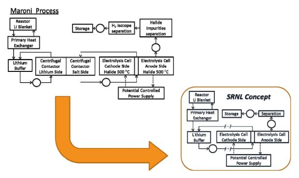
Figure 5. Comparison of the direct LiT electrolysis method with the Maroni process
