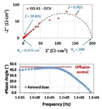
Figure 1. Electrochemical impedance spectroscopy testing of Haynes 230 at 850°C in KCl-MgCl<sub>2</sub>
