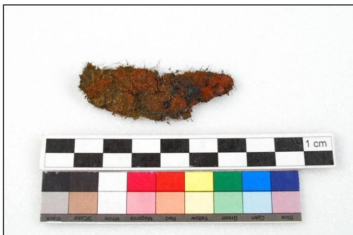
Textile fragment before conservation. Notice the iron corrosion products and an another unidentified material (brown in color) completely covering the wool.
