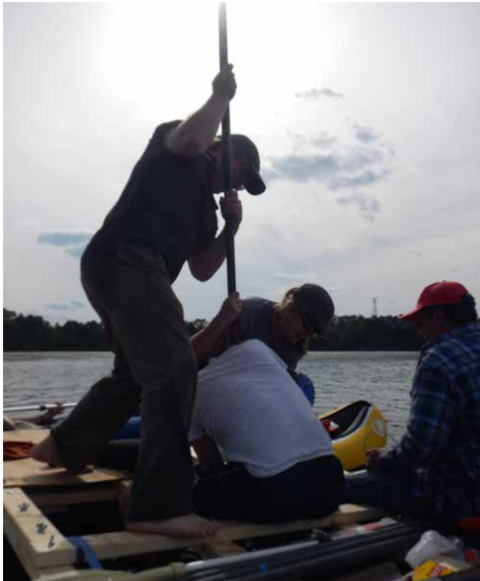
Figure 6: Collecting a sediment core by pushing the core barrel from a floating platform on White Pond. (SCIAA photo by Christopher Moore)
