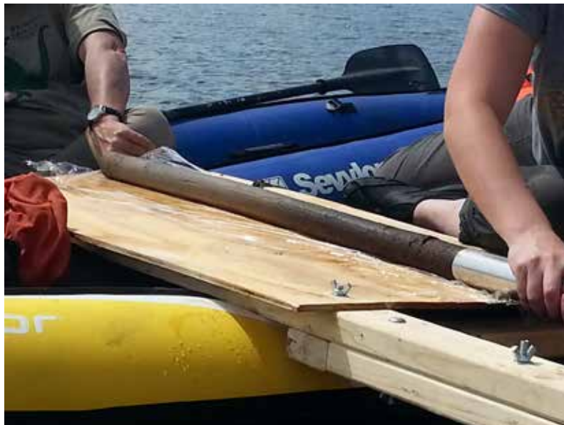
Figure 7: Extracting a core section containing the Pleistocene-Holocene transition. (Note the transition between lighter colored Pleistocene-age silty sediments and darker, organic rich, Holocene-age sediments.) (SCIAA photo by Christopher Moore)
