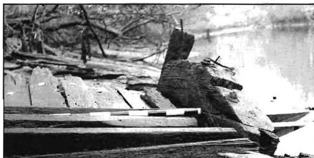
Shaft log on motorized vessel shows shaft hole. (SCIAA Photo)
