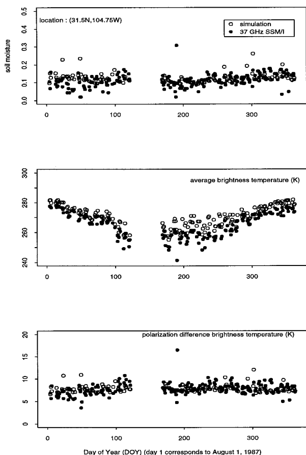
FIG. 9. Good agreement between the simulated and 37-GHz SSM/I brightness temperature-derived soil moisture and average and polarization difference brightness temperature at the location 31.5°N and 104.75°W.
