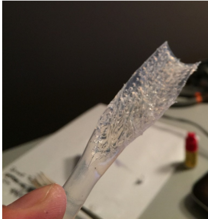
Figure 20. This figure shows the liquid silicone application on deformed wall of the PTFE tubing.
