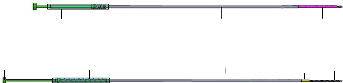
Figure 9. Nasogastric tube in suction position (A) and in cleaning position (B).
