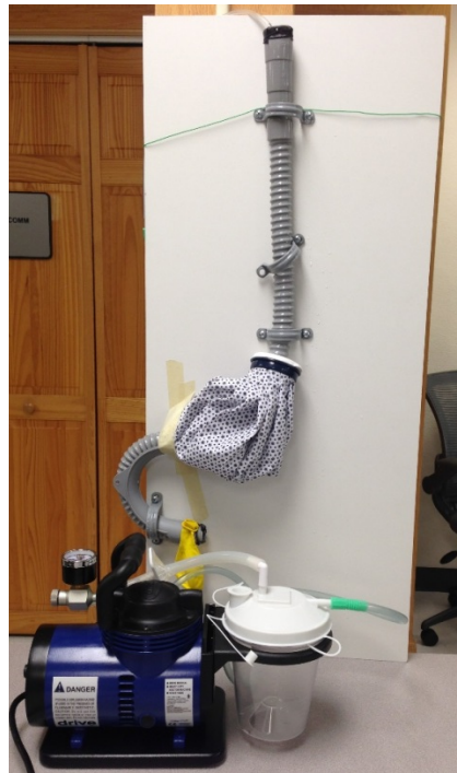
Figure 29. Actual testing setup with pseudostomach, esophagus, and Drive Medical suction machine.
