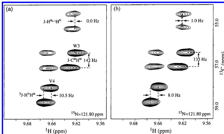
**Figure 1.** Soft HNCA-E. COSY spectra of rubredoxin under (a) isotropic and (b) phage aligned conditions. The  $C^\alpha$  chemical shifts,  $C_i^\alpha$  to  $C_{i-1}^\alpha$  connectivities, and three-bond  $H^N H^\alpha$  scalar coupling constants can be obtained from spectrum (a), and  $C^\alpha-H^\alpha$  dipolar couplings and both inter- and intraresidue  $H^N H^\alpha$  dipolar couplings can be obtained from differences between the measured couplings in these two spectra.
