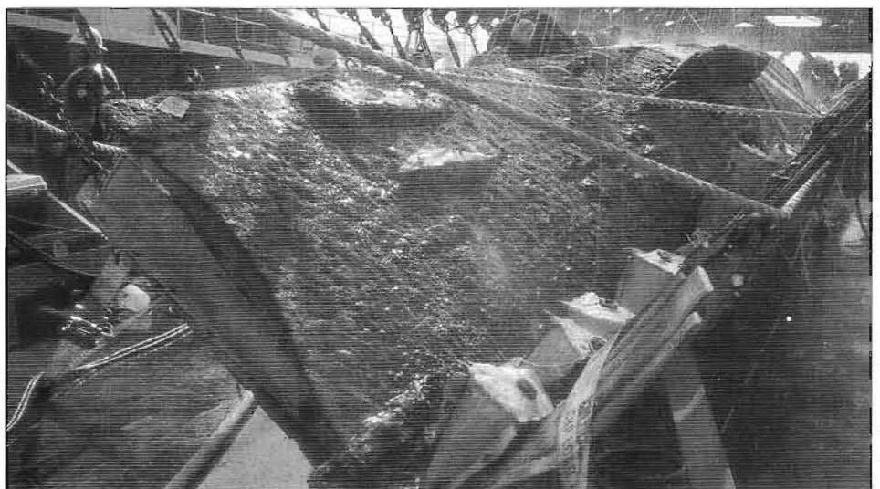
The graceful bow of the Hunley . Note the incurved line of the bow, reminiscent of the bows of dreadnought battleships. (SCIAA photo by Christopher Amer)
