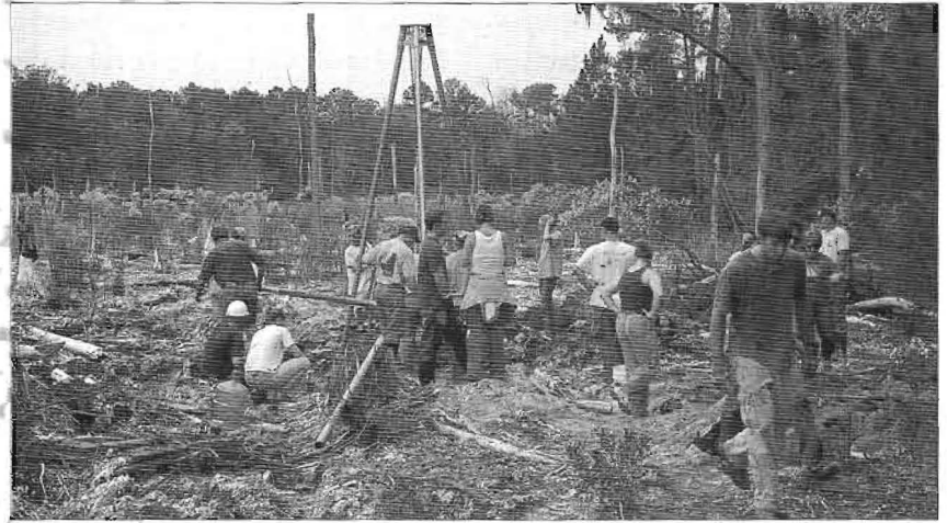
Figure 9: Geology team from USC and Coastal Carolina University vibracoring marsh at the Turnaround site November 2000. (SCIAA photo by Daryl P. Miller)
