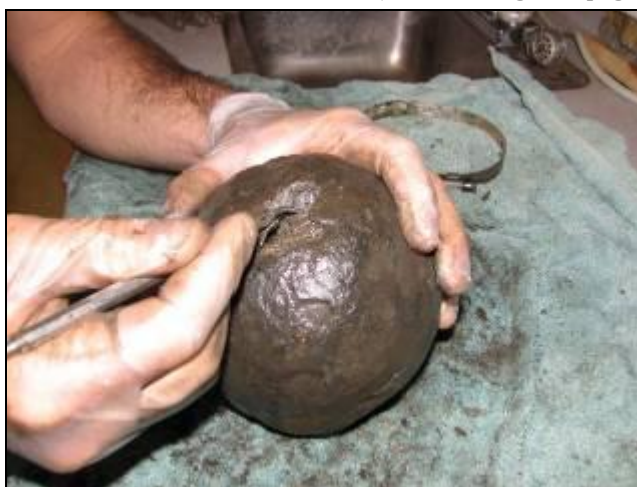
Figure 3 Deep holes must be cleaned to prevent further corrosion
