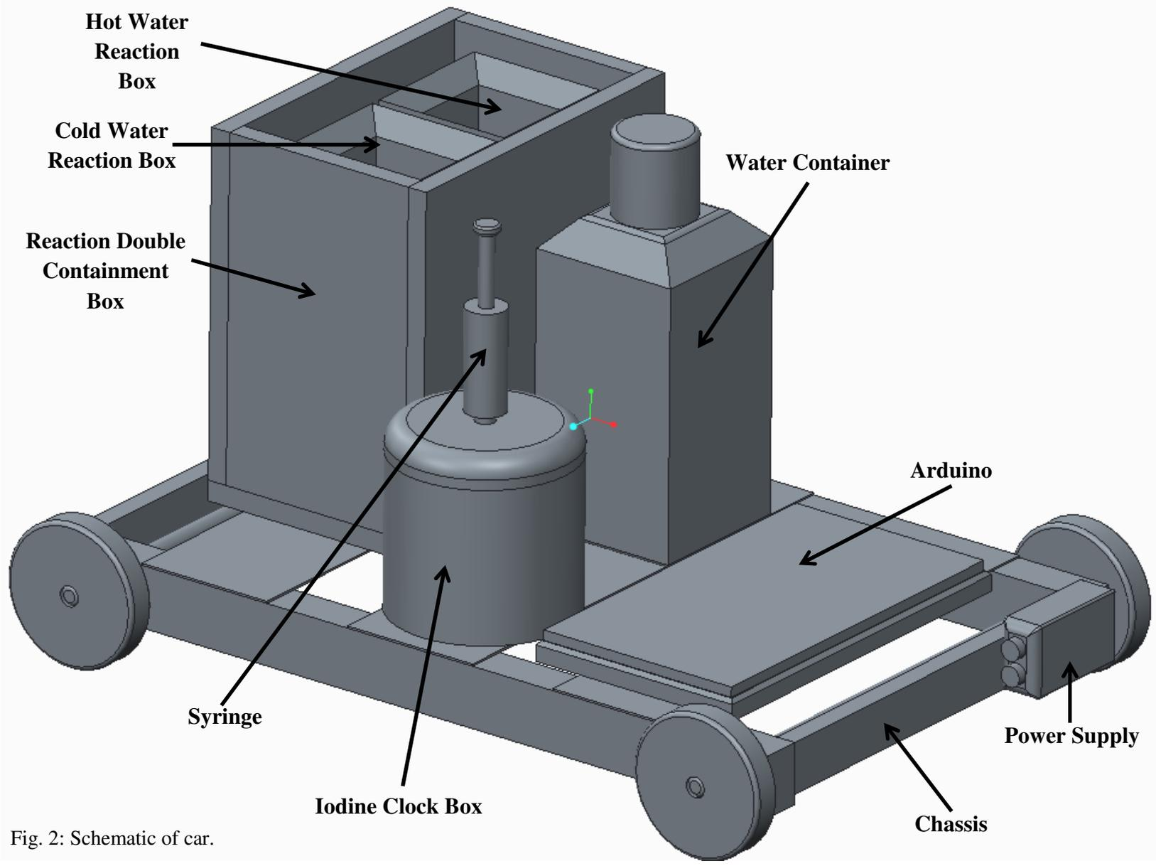
Fig. 2: Schematic of car.
