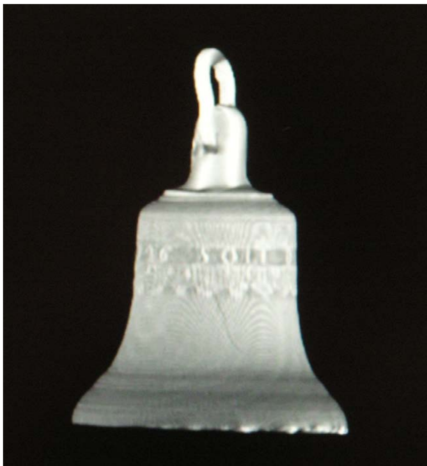
The CAT scan of the 1726 bell revealed a structural defect from the manufacture. (SCIAA photo by Jonathan Leader)
