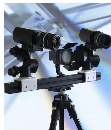
Figure 6: Modern stereo-vision system. Light source is located between the cameras. Cameras are mounted to a rigid cross-bar and can be rotated and translated along bar. Bar is mounted to a sturdy tripod so that the height can be adjusted as needed.
