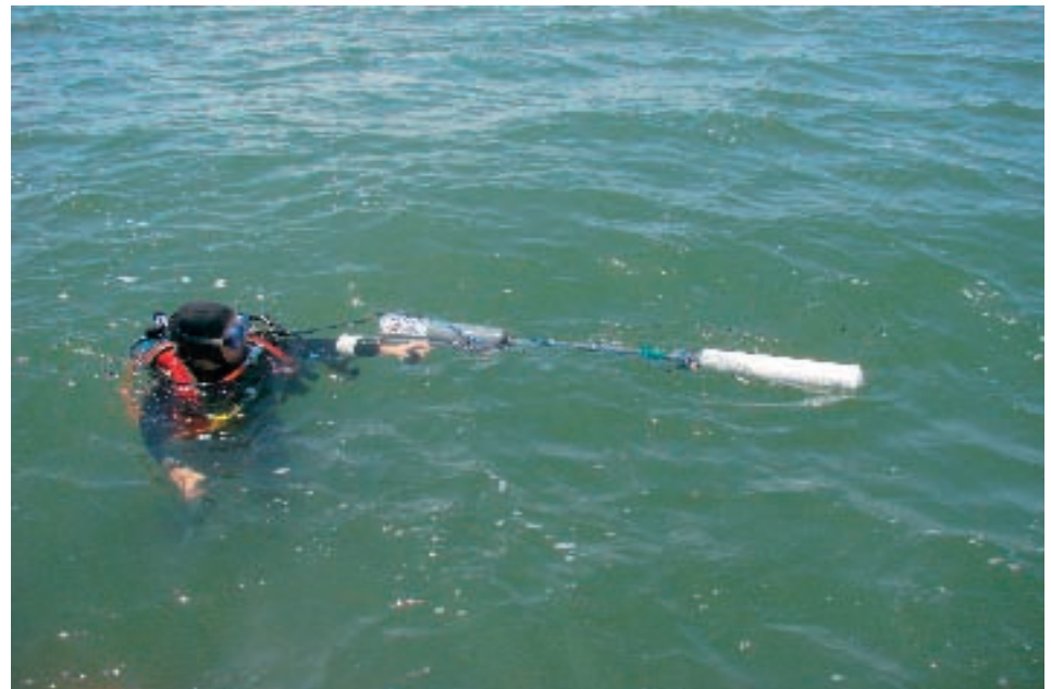
Fig. 5: Emily Jateff handles the hand-held magnetometer at the surface before diving to investigate a target. (SCIAA photo)
